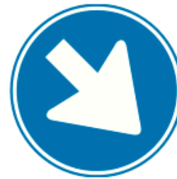
D2 Instruction to all drivers to keep to the right of the sign (or left if arrow is reversed)
